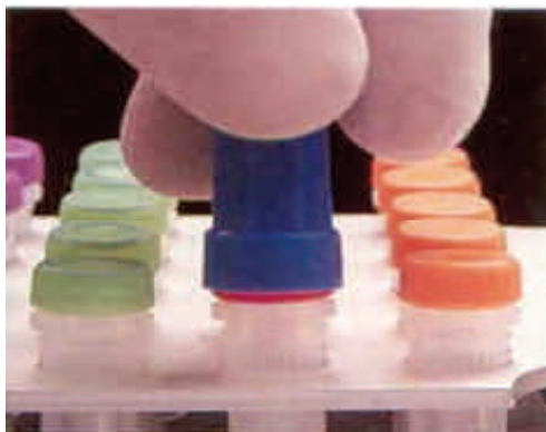
The Micro tube tool's larger end is a socket wrench for Screw-Cap Micro Tubes.
