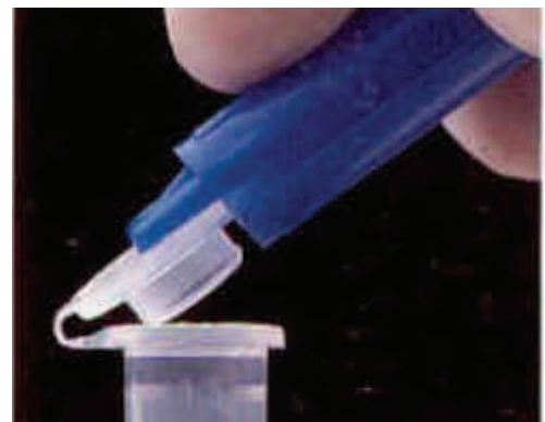
The Micro Tube tool's smaller end is used to open a Snap Cap Micro Tube.
